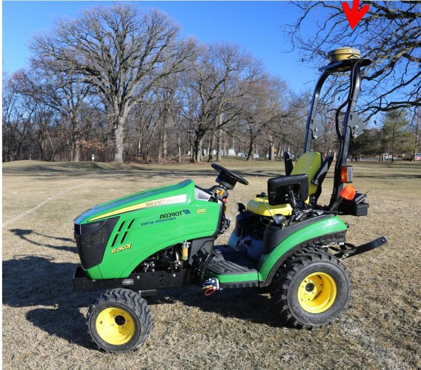
John Deere Sub-Compact Utility Tractor Equipped with Topcon Universal Auto-Steer System
